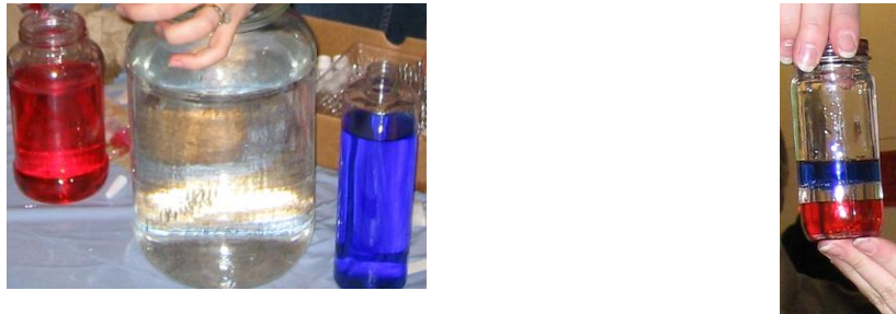
Figure 1. Demonstration of the patriotic pour experiment showing the components used: water, red corn syrup and blue lamp oil.
